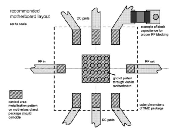
The RF ports comprise a DC blocking capacitor on chip level. The DC connections include a first level of DC decoupling capacitors (typically 120pF) in the package. However, all DC bias ports should be additionally connected to ground with 10nF capacitors at board level to prevent the MMIC from oscillations. These parts should be placed close to the SMD leadless package. If the same bias is required at different DC ports, the lines should only be connected behind these block capacitors.
