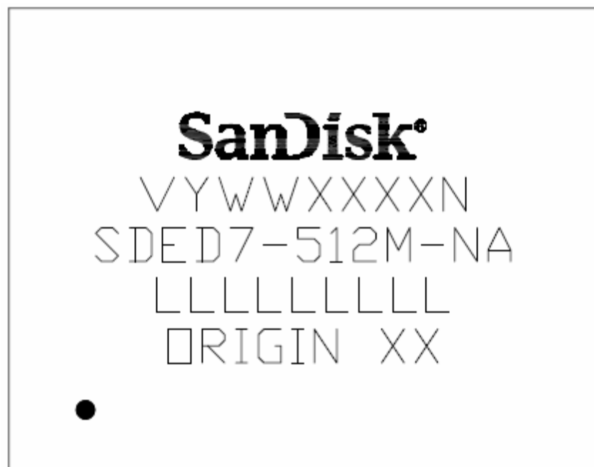
Figure 40: Example of SDED7-512M-NA Product Marking
