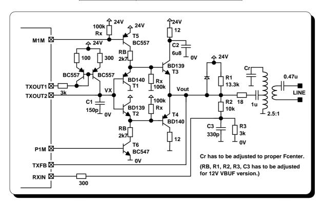
In receive-mode, when the bias-currents are turned off, the base of the two output-transistors are forced by resistors of 100k (Rx) to 0V and Vbuf respectively to guarantee high impedance of the buffer. The current of the pins TxOut1,2 is 0 (VX is floating). Since the receiver-AGC is reacting on signal levels at the RXBPF-filter output, high outband noise-components could give clipping in the first stages of the receiver path. To avoid this, an attenuation of 16dB with R2, R3, C3 is realized.
