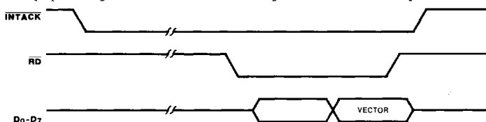
Figure 14. Interrupt Acknowledge Cycle Timing
