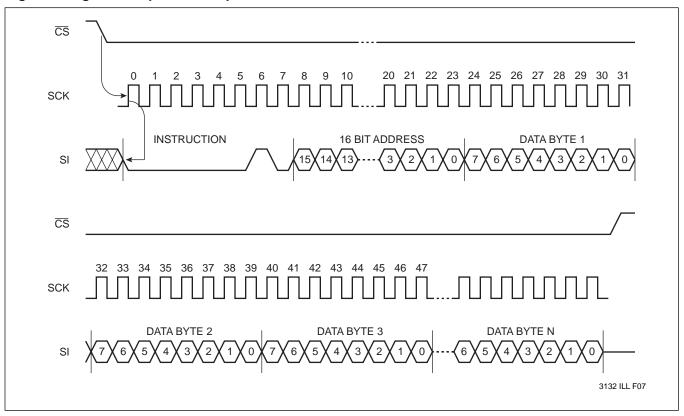
Figure 6. Write Status Register Operation Sequence
