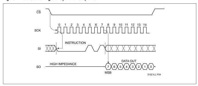
Figure 3. Write Enable Latch Sequence
