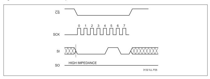
Figure 4. Byte Write Operation Sequence
