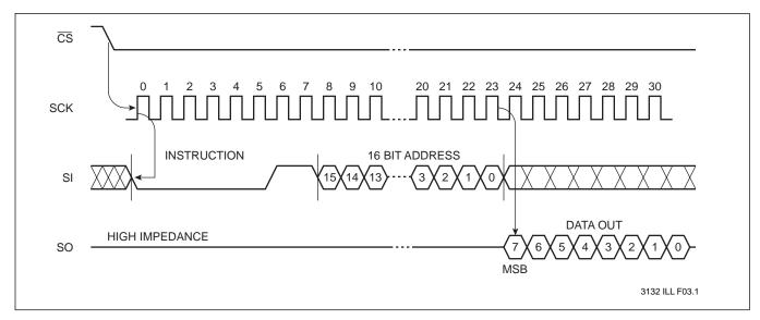
Figure 2. Read Status Register Operation Sequence
