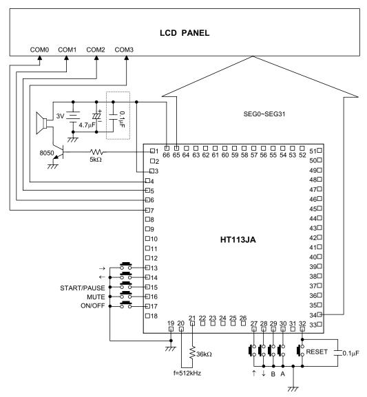
Note: The capacitor in dash block is recommended.
