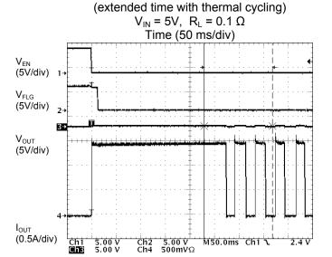
Figure 4. Enable into Short Circuit
