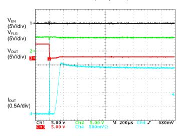
Figure 6. Hot-plugged Short Circuit (extended time with thermal cycling)  $V_{IN}$  = 5V,  $R_L$  = 0.05  $\Omega$  Time (50 ms/div)
