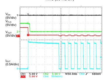
Figure 7. Nuisance Trip Elimination Hot plugged into a capacitive load  $V_{IN}$  = 5V,  $R_L$  = 10  $\Omega$ ,  $C_L$  = 1880  $\mu$ F
