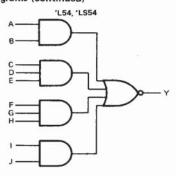
SN54L54... J PACKAGE SN54LS54... J OR W PACKAGE SN74LS54... D, J OR N PACKAGE (TOP VIEW)
