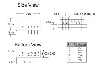
Note: All Pins on a 2.54mm pitch; All Pin diameters are 0.50 mm; all dimensions in mm.
