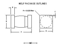
Note: Cathode side of device is indicated by a dark band marked on body.
