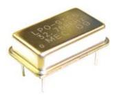
LPO (Low Power Oscillator), such as 32.768 KHz, provides time base for real time clocks. Its low current consumption (only 14 uA for model 3LPO model 7) makes it ideal for battery-operated devices such as data logging and portable test equipments.
