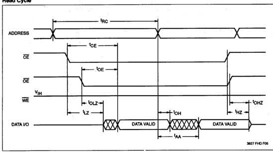
Note: (3) tLZ min., tHZ, toLZ min., and toHZ are periodically sampled and not 100% tested. tHZ and toHZ are measured, with CL = 5pF, from the point when CE or OE return high (whichever occurs first) to the time when the outptus are no longer driven.
