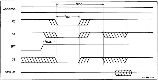
Note: (7) The Recall Pulse Width (tRCP) is a minimum time that NE, OE and CE must be LOW simultaneously. To insure data integrity, NE and CE must remain HIGH after initiation of and through the duration (tRCC) of the Recall operation. During tRCC, OE and WE may go LOW providing the host access to other devices in the system.
