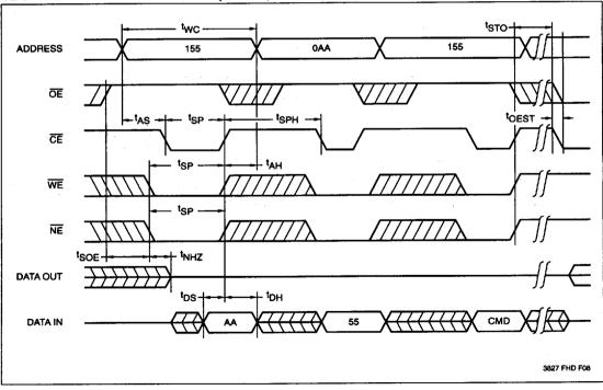
Notes: (5) The Store Pulse Width (tsp) is a minimum time that NE, WE and CE must be LOW simultaneously. To Insure data integrity, NE and CE must remain HIGH after initiation of and throughout the duration (tsto) of the Store operation. During tsto, OE and WE may go LOW providing the host system access to other devices in the system.
