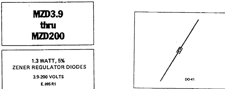
ELECTRICAL CHARACTERISTICS ( $T_A = 25^\circ C$  unless otherwise noted.)  $V_F = 1.5 V$  max,  $I_F = 200 \text{ mA}$ , for all types.
