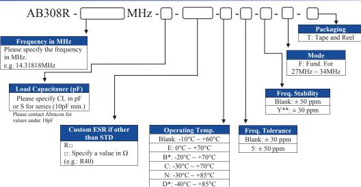
\* Frequency stability:  $\pm$  50 ppm only \*\*Standard Temperature -10°C ~ +60°C, F  $\geq$  6MHz only
