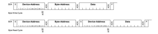
After the AS-Interface slave IC has sent the START condition, the device address is transmitted. This address would allow the selection of a maximum of 8 possible E<sup>2</sup>PROM ICs, is however fixed to 000 by the AS-Interface slave IC. Therefore in the application pins AO...A2 of the E<sup>2</sup>PROM are connected to Uss.
