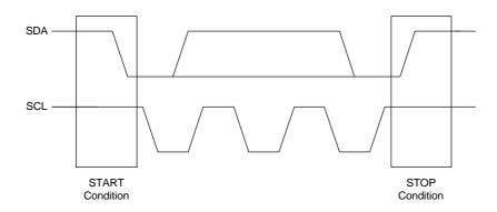
The **START condition** is recognized by the E<sup>2</sup>PROM when a H/L edge arises on the dataline SDA during the high phase of the clock.
