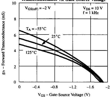
Transconductance vs. Gate-Source Voltage
