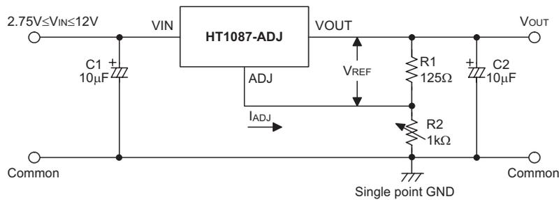
$$V_{OUT} = V_{REF} \left( 1 + \frac{R2}{R1} \right) + I_{ADJ} R2$$
