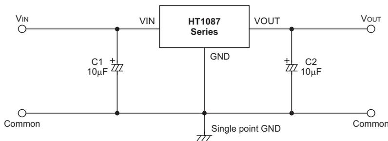
Note: C1 is required if the needed if the device is located far from filter capacitors, the recommended value is 10µF.
