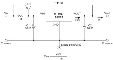
$$R_1 = \frac{V_{BE1}}{I_{REG} - \frac{I_{C1}}{(1+\beta)}}$$
