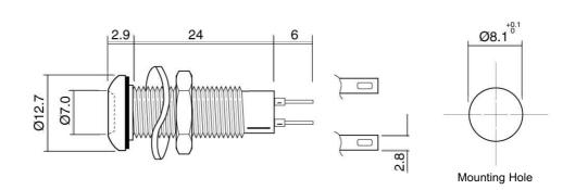
Dimensions in mm (Typical) Not to scale Anode termination indicated by red sleeve Mounting hole to be clean and burr free
