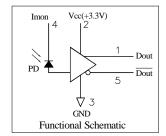
Pin Assignment 1~Dout 2~Vcc 3~GND(CASE) 4~Imon 5~Dout
