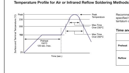
Recommended time and temperature for soldering conditions is specified for the surface and terminal temperature of the polymer tantalum chip capacitors.
