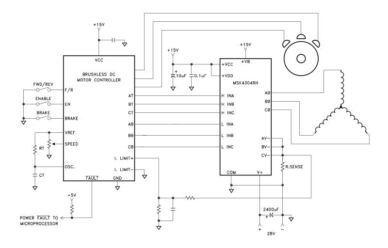
The MSK 4304RH is designed to be used with a +28 volt high voltage bus, +15 volt low power bus and +5 volt logic signals. Proper derating should be applied when designing the MSK 4304RH into a system. High frequency layout techniques with ground planes on a printed circuit board is the only method that should be used for circuit construction. This will prevent pulse jitter caused by excessive noise pickup on the current sense signal or the error amp signal.
