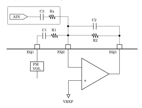
Gain and filter characteristic are adjusted by value of C1, C2, R1 and R2. Gain = R2 / R1. Recommendation of R1 is  $22k\Omega$  and R2 is  $82k\Omega$  (gain = 3.7 times). Cut off frequency f1 and f2 of filter is as follows.
