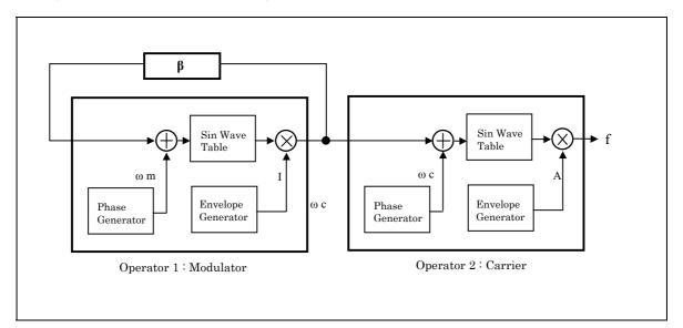
The "Operator" refers to the section where a sine wave is generated and the combination of the operators is called "algorithm". The operator in the front stage is called "modulator" and that in the rear stage "carrier". Each operator is capable of setting the frequency and the envelope waveform. The configuration in the above diagram can be expressed in the formula as follows.
