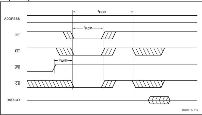
Note: (5) The Recall Pulse Width (t<sub>RCP</sub>) is a minimum time that  $\overline{\text{NE}}$ ,  $\overline{\text{OE}}$  and  $\overline{\text{CE}}$  must be LOW simultaneously to insure data integrity,  $\overline{\text{NE}}$  and  $\overline{\text{CE}}$ .
