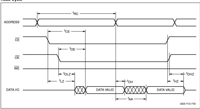
Note: (3)  $t_{LZ} \min_{\cdot}, t_{HZ}, t_{OLZ} \min_{\cdot}, \text{ and } t_{OHZ} \text{ are periodically sampled and not 100% tested. } t_{HZ} \max_{\cdot} \text{ and } t_{OHZ} \max_{\cdot} \text{ are measured, with } C_{L} = 5pF, \text{ from the point when } \overline{CE} \text{ or } \overline{OE} \text{ return HIGH (whichever occurs first) to the time when the outptus are no longer driven.}$
