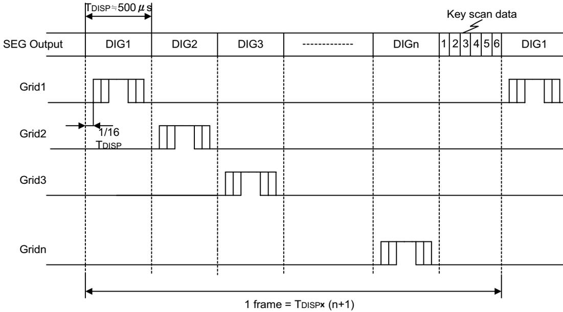
One cycle of key scanning consists of one frame, and data in a 6x 4 matrix is stored in RAM.
