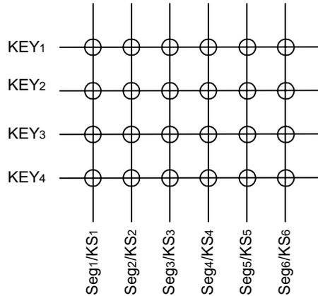
The data of each key is stored as illustrated below, and is read with the read command, starting from the least significant bit.
