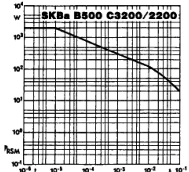
Fig. 7 Rated reverse power dissipation vs. time
