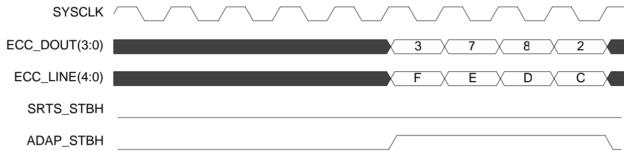
Figure 106 Channel Status Functional Timing
