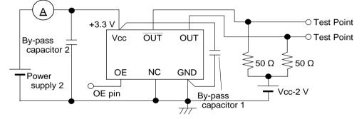
\* The lines from OUT and  $\overline{\text{OUT}}$  pin are same length.
