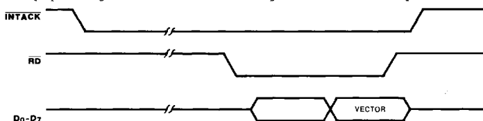
Figure 14. Interrupt Acknowledge Cycle Timing
