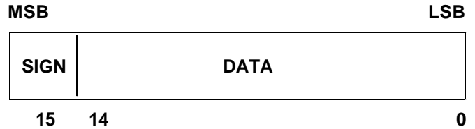
Figure 31a. Single 16-bit Precision Fixed-Point Data
