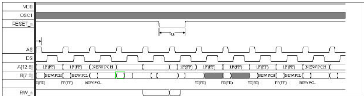
Figure 16. Power-On-Reset and RESET\_n Timing
