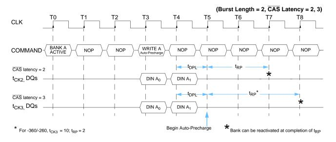
Similar to the Read Command, a Write Command with auto-precharge can not be interrupted by a command to the same bank. It can be interrupted by a Read or Write Command to a different bank, however. The precharge function will begin with the new command. The bank may be reactivated after  $t_{RP}$  is satisfied.
