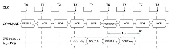
\* Bank A can be reactivated at completion of t<sub>RP</sub>
