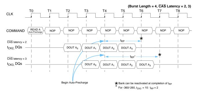
Although a Read Command with auto-precharge cannot be interrupted by a command to the same bank, it can be interrupted by a Read or Write Command to a different bank. If the interrupting command is issued before auto-precharge begins then the precharge function will begin with the new command. The bank being auto-precharged may be reactivated after the delay  $t_{\rm RP}$ .
