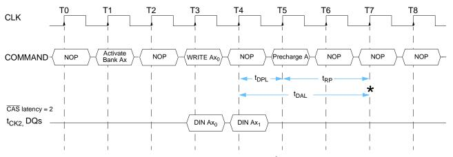
$\bigstar$  Bank can be reactivated at completion of  $t_{DAL}$
