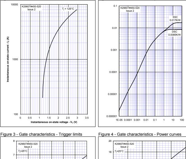
Figure 1 - On-state characteristics of Limit device
