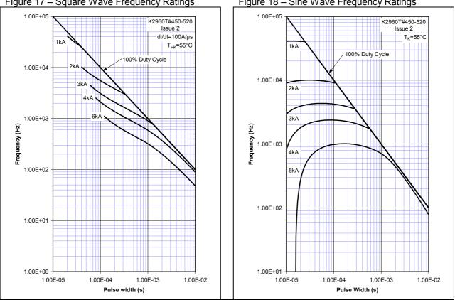
Figure 17 – Square Wave Frequency Ratings
