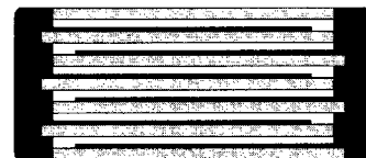
Extended metallized film design
