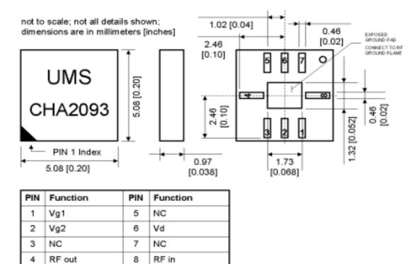
"Please note that PIN 1 is located in the lower left corner of the package (front-side view) for all SMD-type packages from United Monolithic Semiconductors. It is indicated by a triangle on the package lid. Starting with PIN 1 the other pads are numbered counter-clockwise (front-side view). ATTENTION: The dot on the backside of the package (i.e. side with metallic pads) is just for fabrication purposes and does NOT indicate the location of PIN 1."
