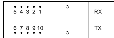
Figure 1. 1417K4A Transceiver, 10-Pin Configuration, Top View
